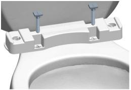
3) Curved edge facing the bowl, align the correct mounting holes and slide the bolts thru the base and into the ceramic
