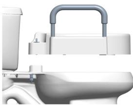
5) Slide the arms in, depress button to lock 6) Align the back of the seat with the Mounting Base and slide the seat on
