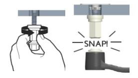
4) Finger tighten the Snap 2 Secure nuts. Use a 5/8" wrench, tighten until the Installation Heads snap off
