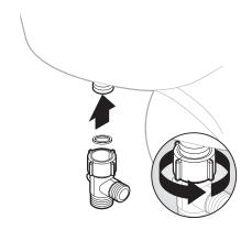
4. Connect water supply line coming from the wall to bottom of T-valve. Connect cold water supply only. If your water supply line is rigid, you may need to replace with a flexible hose line.
