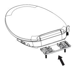
4. Place bidet seat on bowl, adjusting seat front-to-back and side-to-side for proper fit.
