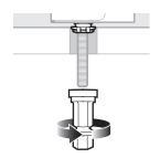
Holding seat centered on bowl, tighten the Stay-Tite® nut until lower portions SNAP OFF to prevent over-tightening and will NEVER LOOSEN.
