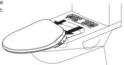
After cleaning, slide closed seat back onto the mounting plate to reinstall.
