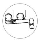
install splice mounting brackets tray on the bidet body
