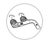
8. Insert the rubber non-slip mats to the bottom of the bidet.
