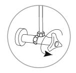
12. Slowly turn the water supply valve back on, check for leaks, and test the unit for functionality.
