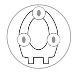
14. If necessary, place the bumpers on the underside of your toilet seat as indicated above.
