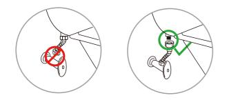
Please be advised that the provided T-Valve should be installed at the fill valve under the toilet tank, NOT down at the water supply coming from the wall.
