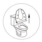
1. Remove the existing toilet seat by locating the bolts and nuts, typically under a plastic cover, and removing them first.
