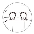
10. Place the bidet on the toilet with the mounting brackets over the bolt holes and make any needed adjustments to make sure the bidet is centered on the toilet.
