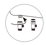
4. Connect the 7/8" T-Valve to the toilet fill valve where you just removed the water hose from.
