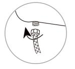
3. Disconnect the water hose from underneath the toilet tank.
