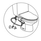
12. Connect the hose from step 6 to the bidet water connection underneath the handle of the Wellspring 100.
