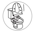
11. Place the toilet seat back on the toilet over the bidet and secure the bolts down so that the seat and bidet attachment are stable.
