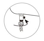
5. Attach the water supply hose that comes from the water shut off to the bottom of the T-Valve.
