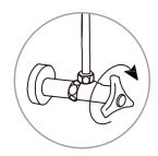
2. Close the water supply valve and flush the toilet completely so that there is little to no water left in the toilet tank.
