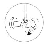
13. Slowly turn the water supply valve back on, check for leaks, and test the unit for functionality.
